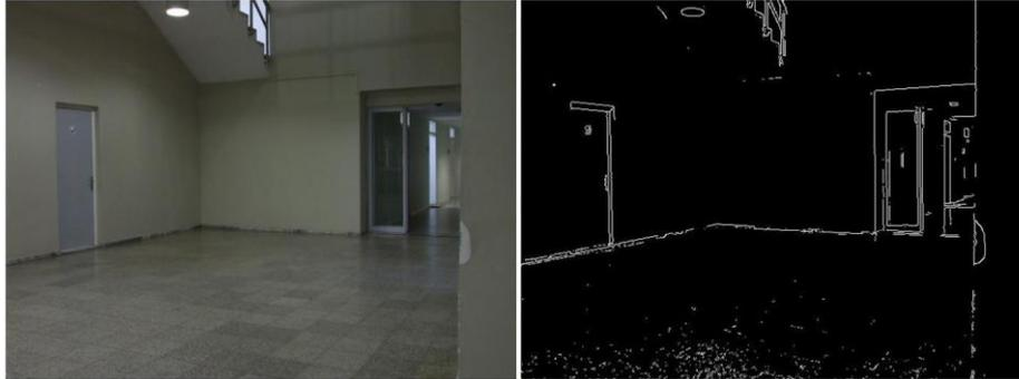
**Fig. 2.** Results of Canny Filter applied on the raw corridor image
