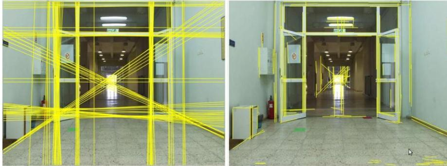
**Fig. 3.** Standard Hough Transformation (left) and Progressive Probabilistic Hough Transformation (right)
