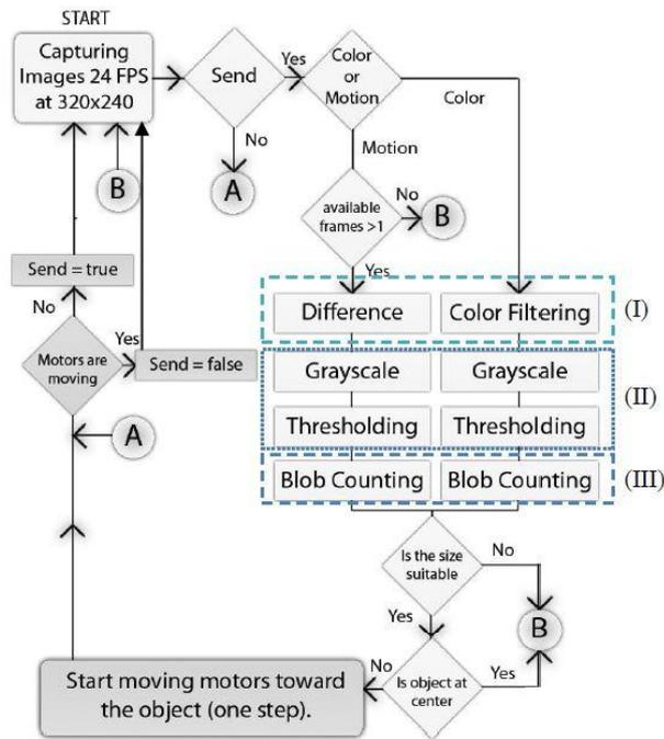
**Fig. 2.** The main loop of detection and movement: (I) Feature extraction, (II) Reducing calculation redundancies, (III) Object detection.
